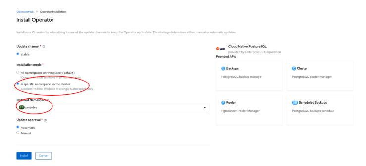
As a result, the operator will be visible in the selected namespace only. You can verify this from the Installed operators page:
