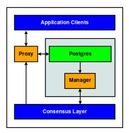
The consensus layer is an external entity where HARP Manager maintains information it learns about its assigned Postgres node, and HARP Proxy translates this information to a valid Postgres node target. Because HARP Proxy obtains the node target from the consensus layer, several such instances can exist independently.
